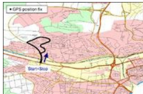
Figure 9: Short course driven in Ulm, Germany, for testing the HTL computation. only 1-sigma level.
